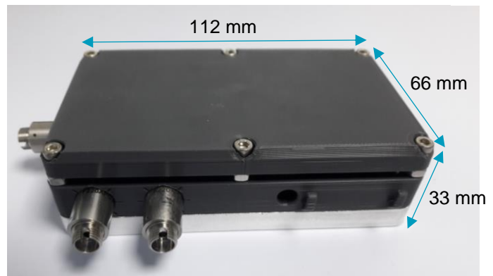
Prototype device with measurements (130 x 90 x 32 mm when including protruding spectroscopy components). Mass = 280 grams.
