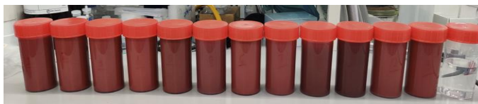
Fig 4: Cu ink produced at larger scale in a continuous flow reactor
